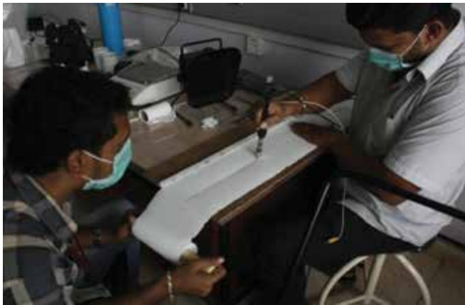
Process of cutting Oxygenator fiber mat to the required size.
