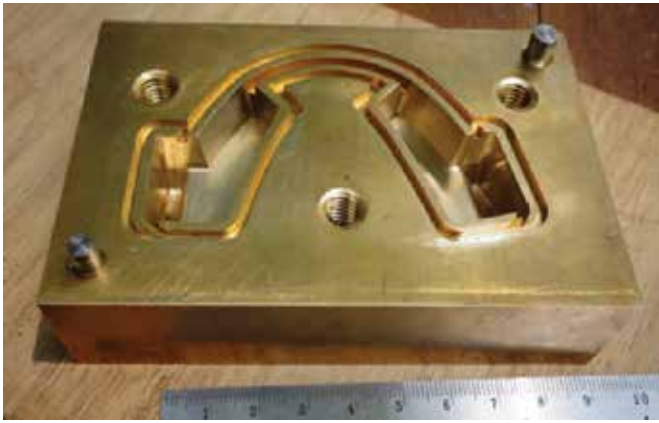
5. Executed the brass top and bottom mould cavity cam portion machining work to the Mandibular advancement Device project.
