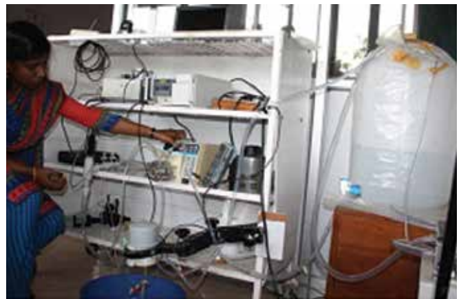
Experiment for estimation of Gas transfer rate
