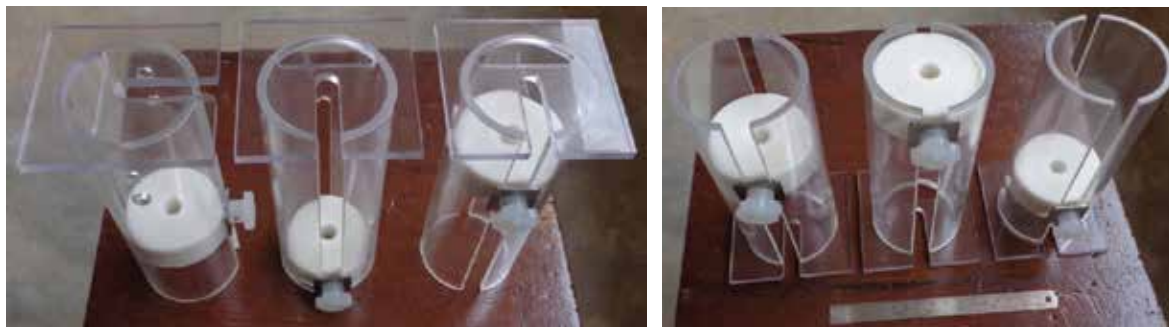
14. Designed and completed 3 sets of Rat Restrainer to Sleep Disorder Research Lab.
