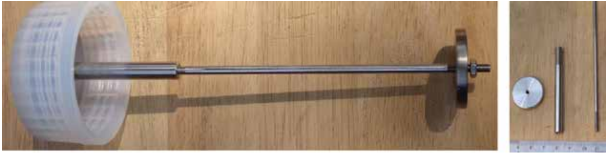
1. Designed and completed the machining of Spinner flask scaffold fixture to TEM lab.
