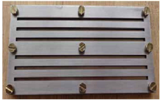
6. Designed and fabricated the 2mm channel S.S. mould to Dental Products lab.
