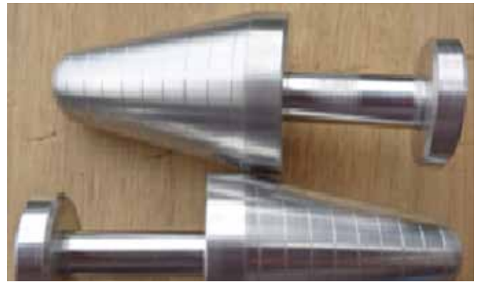
8. Designed and completed the machining of Conical Valve sizer to Hospital wing.
