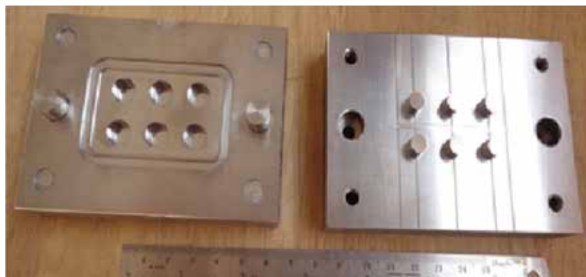
12. Designed and completed the machining of S.S. mould for moulding a multi cavity specimen holder to POP lab.
