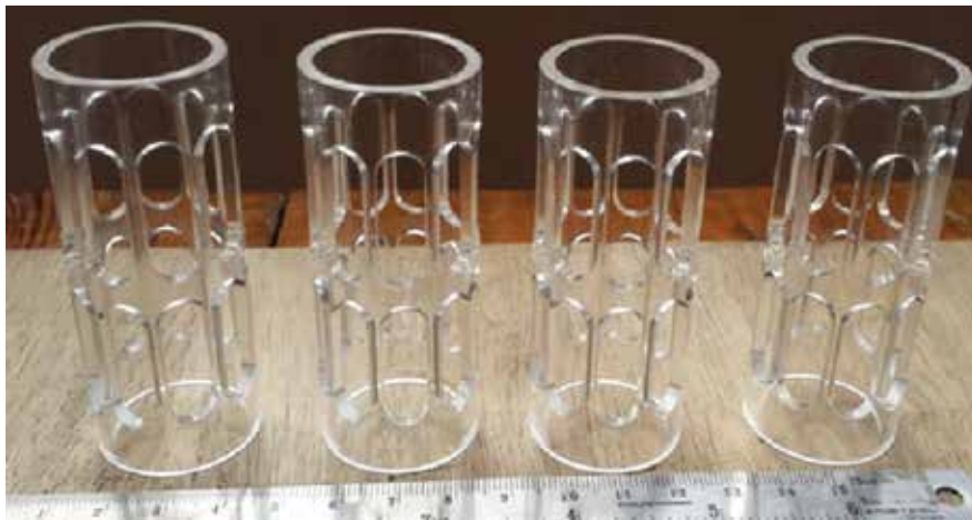
11. Executed the machining of outer shell, inner shell, potting cap, inner tube, cone and inner bottom part components for the Gas exchanger unit of Paediatric oxygenator Project of MPL.
